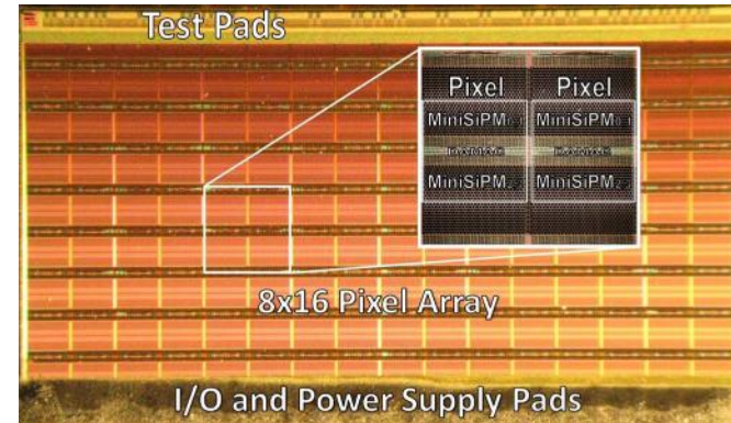
8x16-pixel (92k SPADs) 130nm CIS
